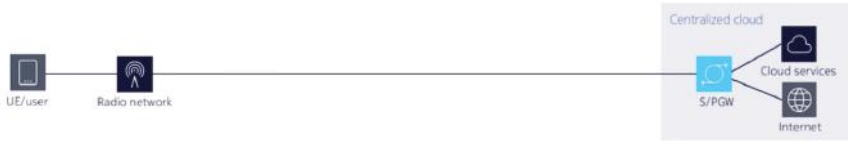
Figure 6. 4G LTE data plane in the cloud with SGW/PGW integrate control and data plane functions. 8
